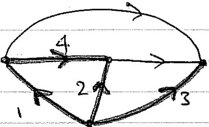
this defines a loop for which we can write KVL.
